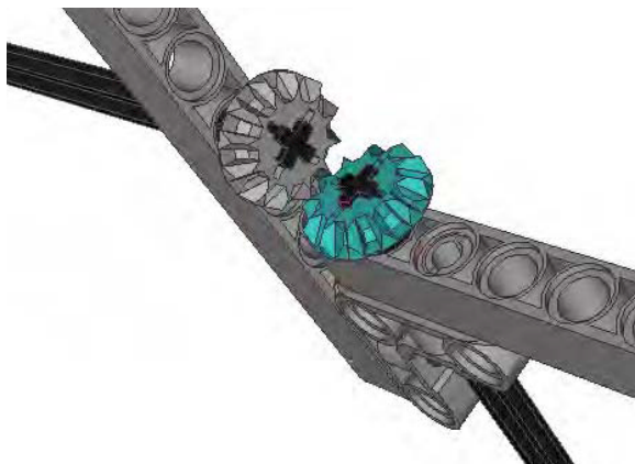
Figure 2–6. Bevel gears work well in tight areas but can only be paired up with other bevel gears.
