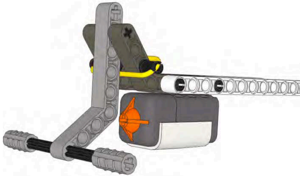
Figure 7-3. A single Touch Sensor bumper assembly
