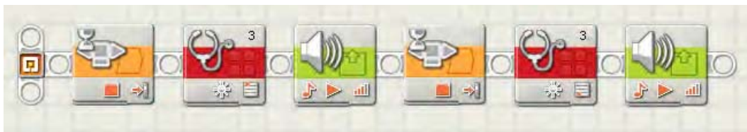
Figure 5–3. A simple NXT-G calibration program
