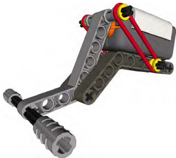
Figure 7-8. A release state bumper that, when pressed, releases the the NXT Touch Sensor instead of pressing it
