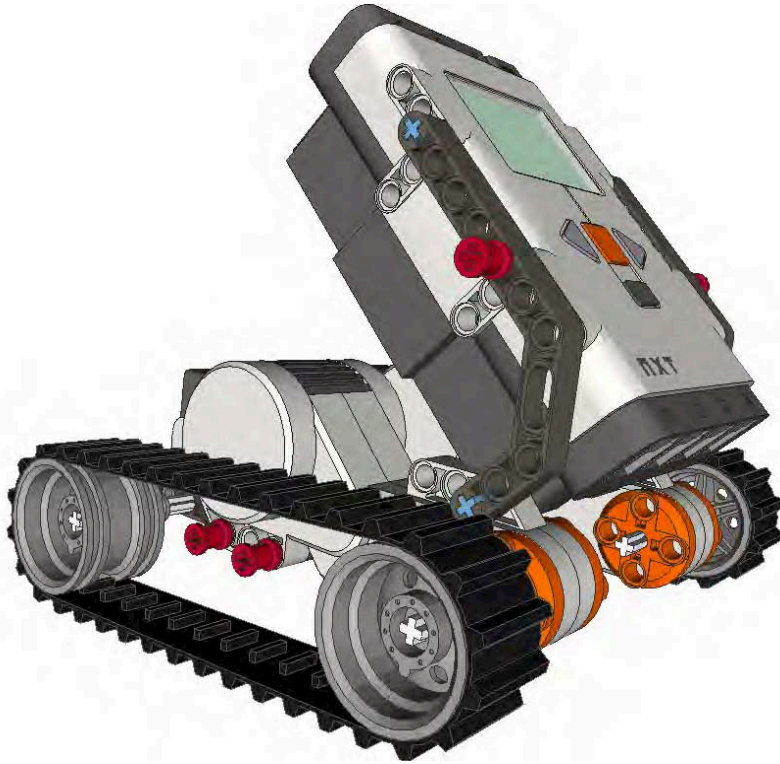
Figure 2-24. A tracked robot
