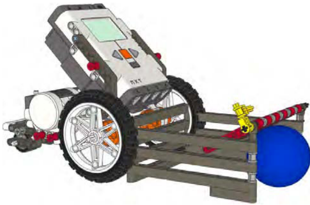
Figure 8-14. As the robot moves forward, the ball pushes its way into the attachment.
