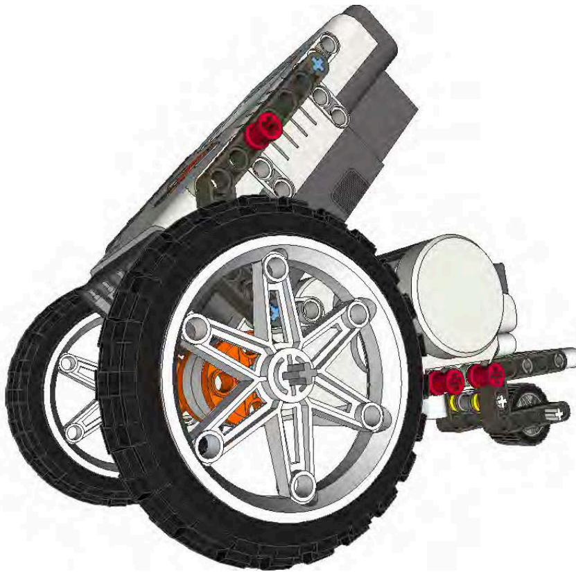
Figure 2–21. A three-wheeled robot with a caster wheel on rear
