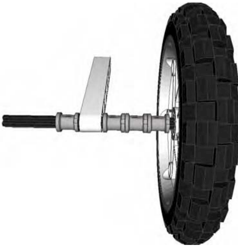
Figure 2-18. Multiple bushing spacing on a wheel axle, moving the wheel further from the chassis causing more friction
