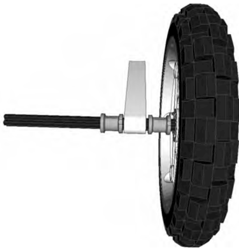
Figure 2-17. Single bushing spacing on wheel axle
