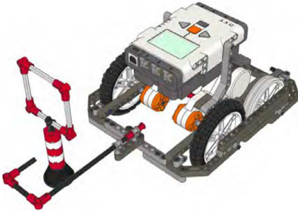
Figure 8-4. A hook attachment moving into place behind the scoring object
