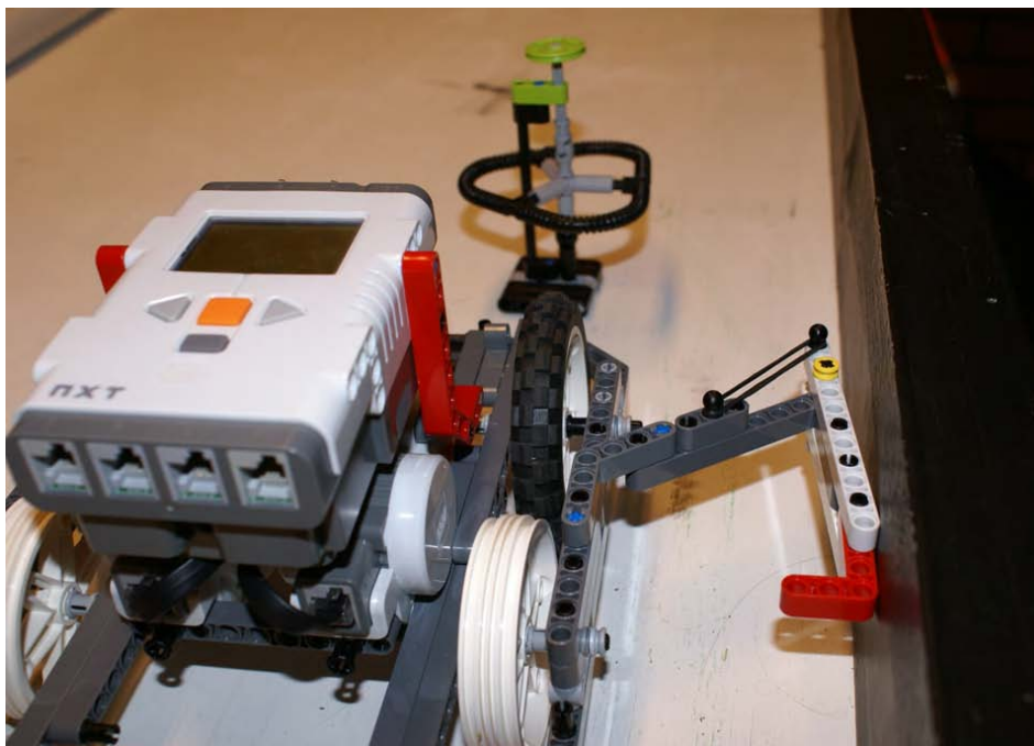
Figure 8–18. A flipper compressed with the game table wall
