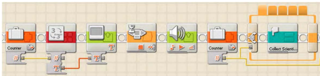
Figure 11-4. The simple sequencer with feedback to the user added such as tones and displays
