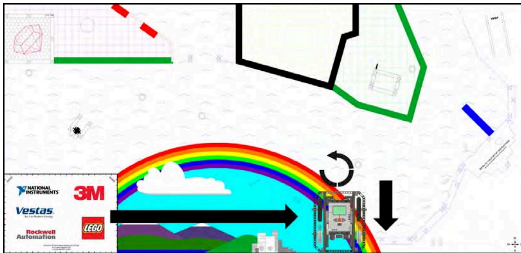
Figure 6–5. The path that the robot follows as it follows the code in Figure 6–4: After making the 90-degree turn, the robot backs up and squares with the wall.
