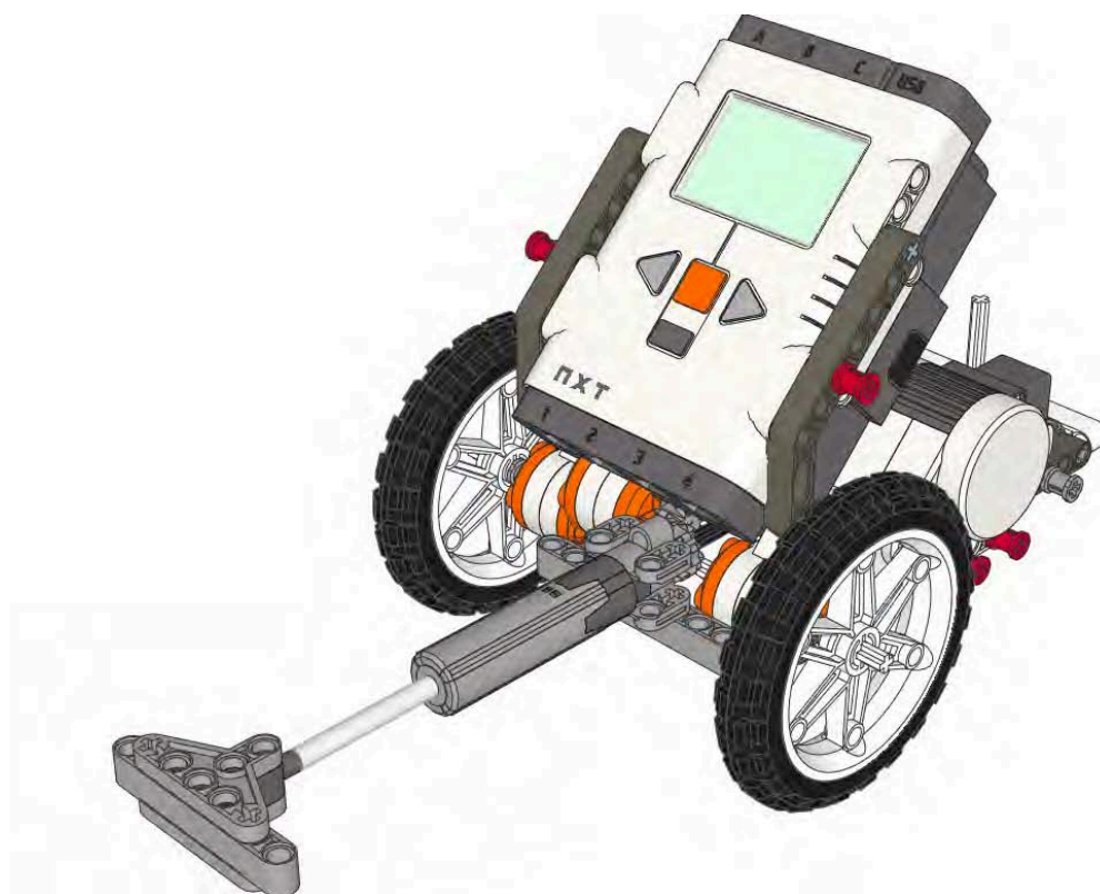
Figure 9-13. LEGO Power Functions actuator mounted to a robot as a pushing power attachment.
