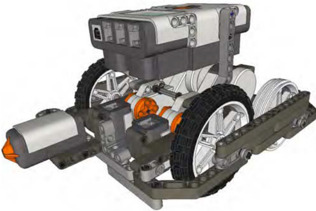
Figure 7-2. DemoBot with single Touch Sensor installed
