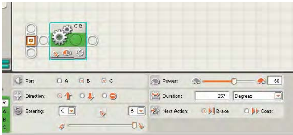
Figure 4-4. A Move block being set to pivot the DemoBot 180 degrees by using the value of 257.4 as the Duration and the steering set to the far right.
