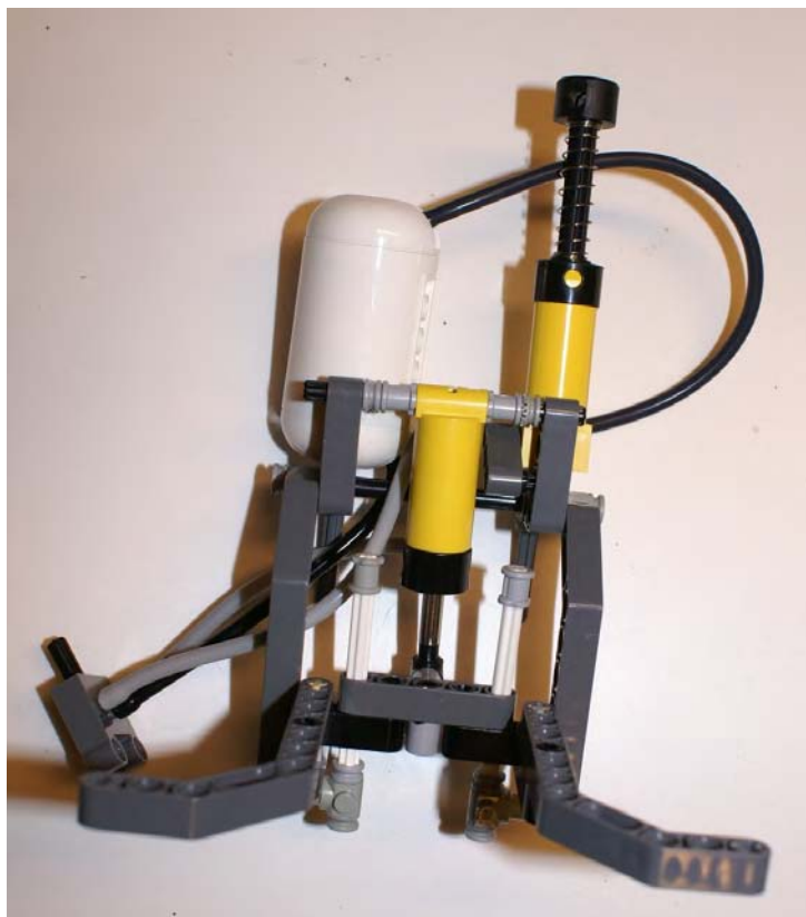
Figure 10–11. A robot's lifting attachment using pneumatics
