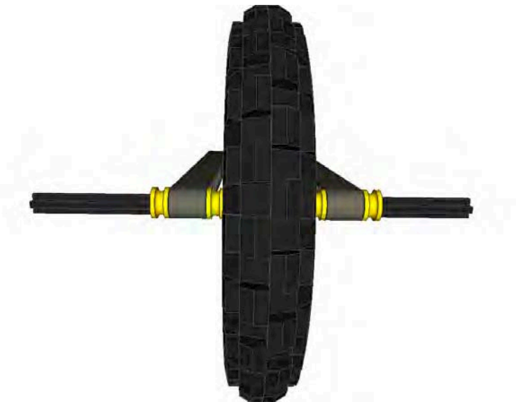
Figure 3–4. With the axle and wheel supported evenly on both ends, the friction is reduced drastically, and you get a much stabler drive system for the robot.
