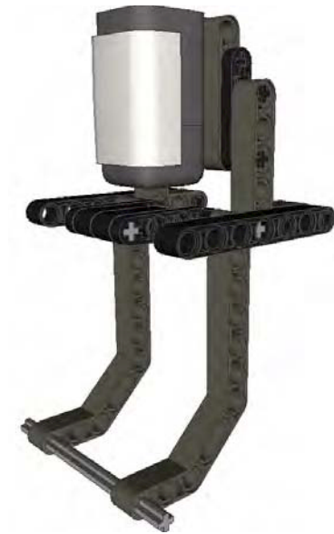
Figure 7-11. A Light Sensor being used to detect touch by a bumper that blocks the Light Sensor's path with black beams
