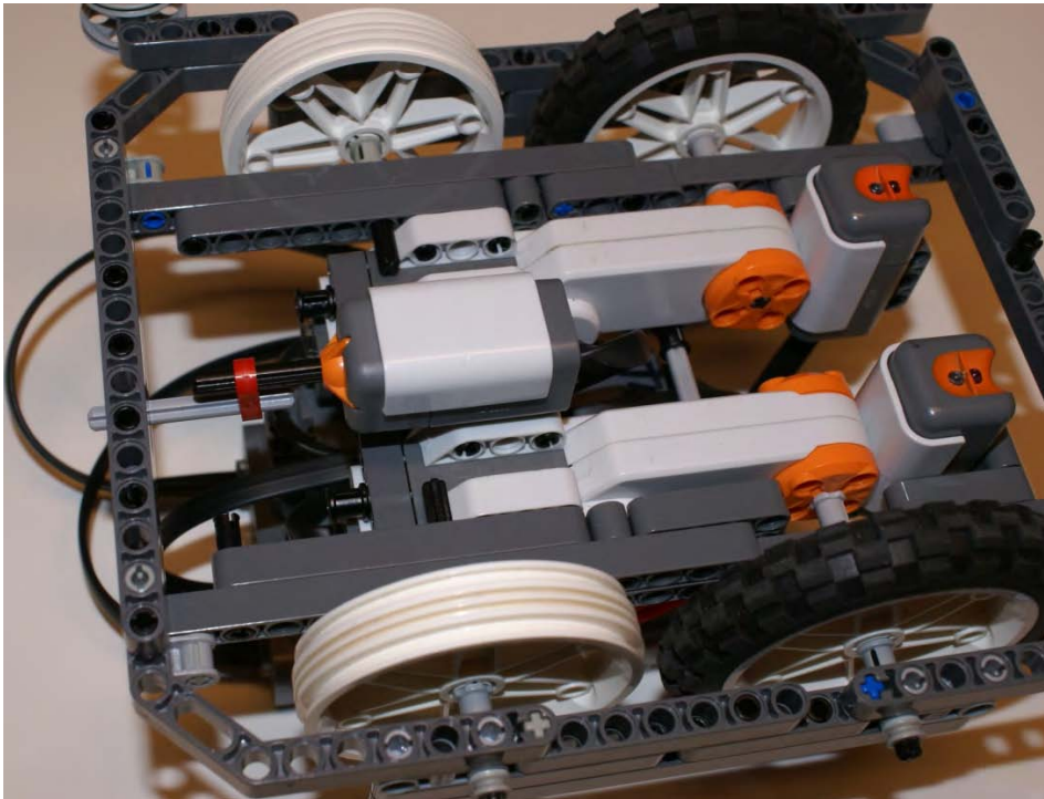
Figure 11–1. DemoBot with rear facing touch sensor installed
