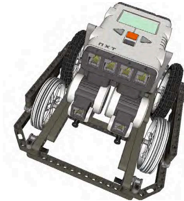
Figure 6-1. DemoBot has a flat rear surface on the chassis to allow for flush contact with the wall when squaring up.
