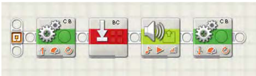
Figure 3–18. This motor matching machine NXT-G program runs the motors forward, stops, resets motors, plays a tone, and then runs the motors backward.
