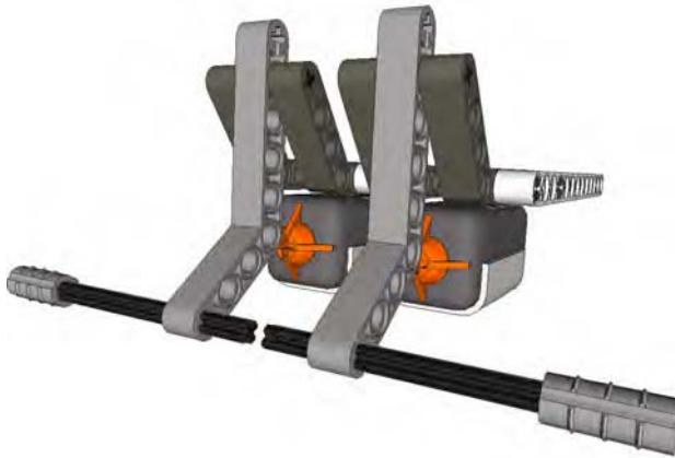
Figure 7-4. A double Touch Sensor bumper assembly
