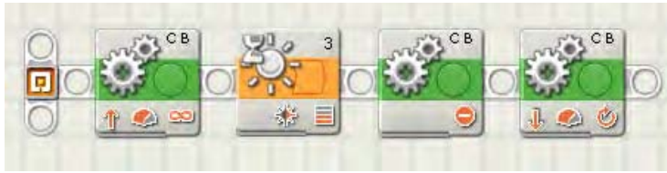
Figure 7-13. NXT-G code using a Light Sensor as a touch detector
