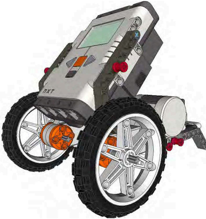
Figure 2-20. A two-wheeled robot with skids in the rear for balance
