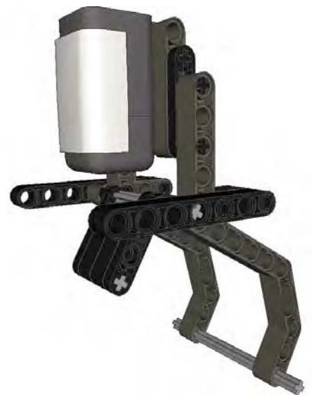
Figure 7-12. With the bumper pushed the black beams are removed from the view of the Light sensor.
